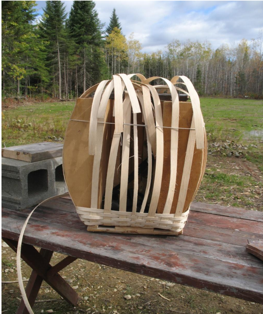
Figure 7. Weaving the Sides of a Pack Basket. In this picture you can see the mold inside the basket, the stand (very bottom of basket), and the first few rows of weaving up the side of the basket.
